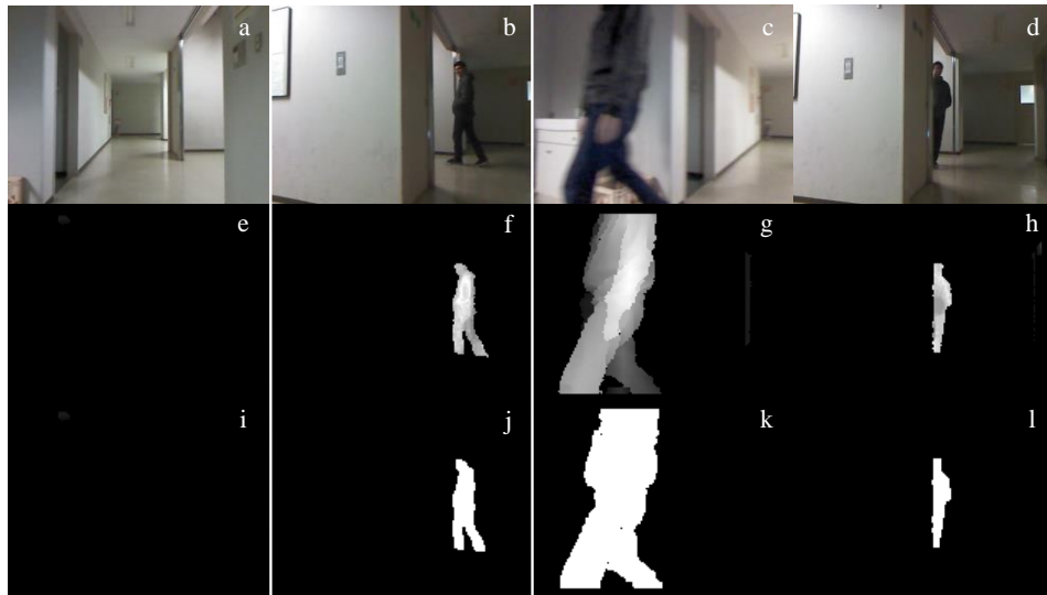
Figure 9: (a) sample image without subject or novelty, (b-d) sample images with subject or novelty representing different conditions such as subject visibility or occlusion and illumination changes, (e-h) space-based saliency maps of the scenes in (a) to (d) respectively, (i-l) extracted novelty regions from saliency maps in (e) to (h)
