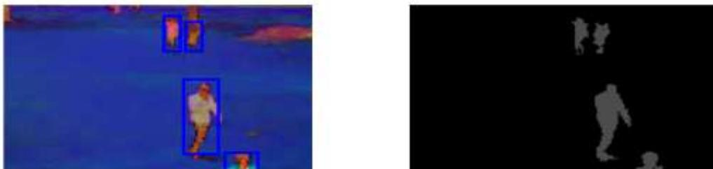
Figure 4: Correct Human Classification and shadows completely removed
