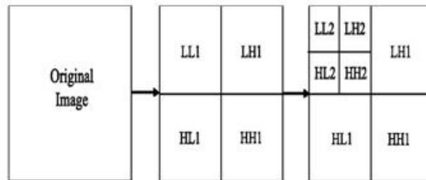
Figure 2: Level 2D – DWT
