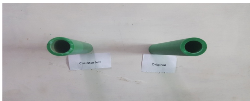
Figure 4. showing both original and counterfeit KAWSAR company pipes. Counterfeit pipes are identified form the color which is slightly different then original one and its gauge is 3mm where as original pipe gauge is 4mm.
