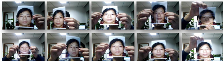
Figure 19. Illustration of different photo-attacks (from left to right) [14]: (1) move the photo horizontally, vertically, back and front; (2) rotate the photo in depth along the vertical axis; (3) the same as (2) but along the horizontal axis; (4) bend the photo inward and outward along the vertical axis; (5) the same as (4) but along the horizontal axis.
