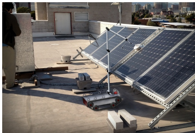
Figure 1: Prototype of the robot Helios with the folding telescopic support of the vision system consisting of four cameras and a noninvasive laser.
