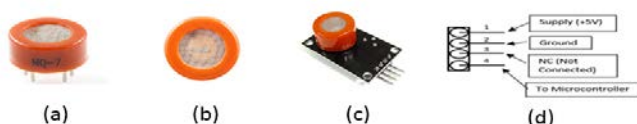
Figure 2. Sensor (a) front view, (b) top view, (c) module and (c) pin configuration
