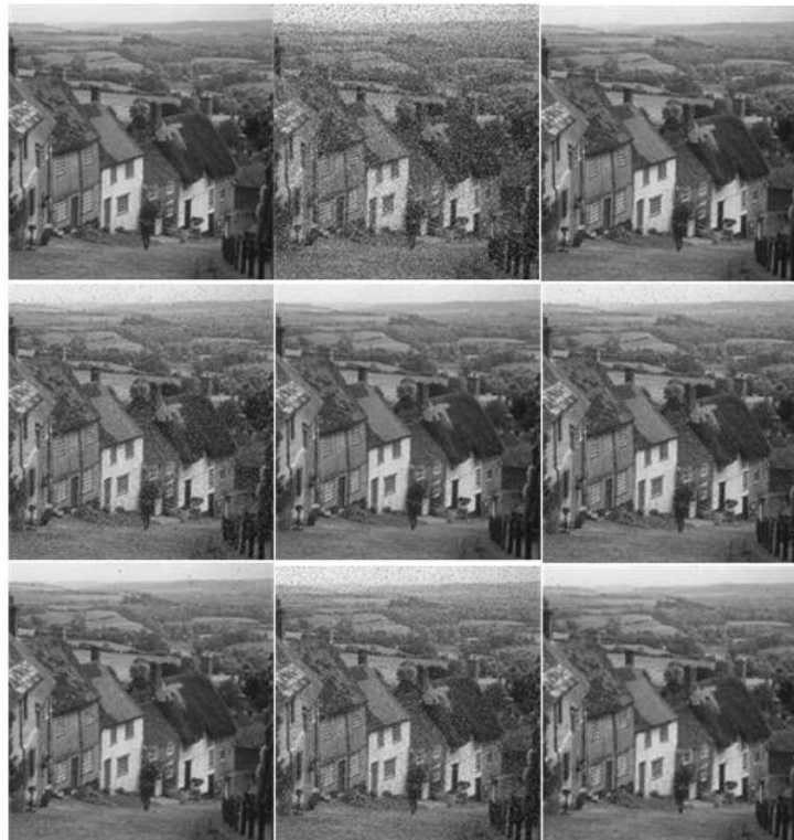
Figure 3: Experimental result with Gold Hill image (a) standard Gold Hill image, (b) noisy image with 30% impulse noise, Restoration result by corresponding (c) FIRE[16], (d)BDND[17], (e) DWM, (f) LUO, (g) FMEM, (h)SAM, (i) PROPOSED METHOD filters.
