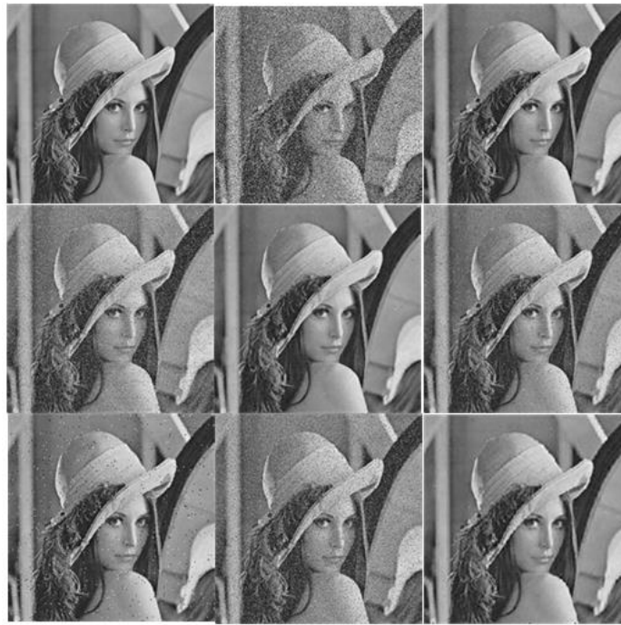
Figure 2: Experimental result with Lena image (a) standard Lena image, (b) noisy image with 30% impulse noise, Restoration result by corresponding (c) FIRE[16], (d) BDND[17], (e) DWM, (f) LUO, (g) FMEM, (h) SAM, (i) PROPOSED METHOD filters.
