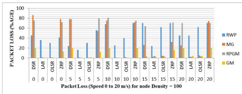
Figure 11: Packet Loss at Node Density 100, with speed varying from 0 to 20 m/s
